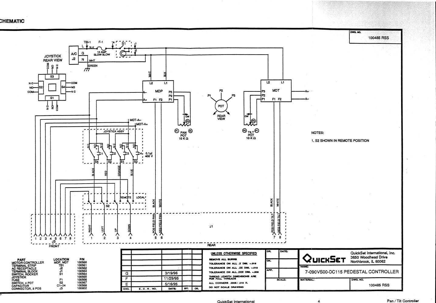
Pan / Tilt Controller Model 7-090VS00-DC115
